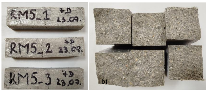
Figure 3: RM5 mortar specimens: a) after 7-day flexural strengths examination, and b) before compressive strength examination
