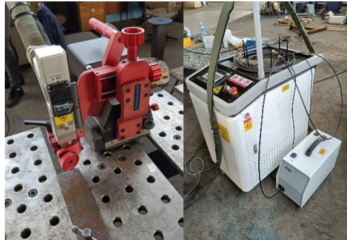
Figure 1. Experimental setup: a) welding tractor; b) welding device
